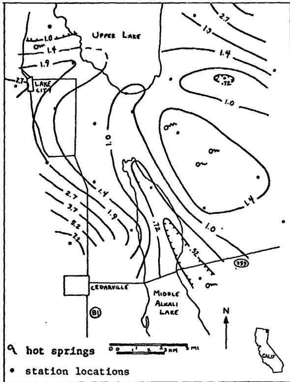
Fig. 1 Audio-magnetotelluric apparent resistivity map at 7.5 hertz, Surprise Valley, California KGRA. Logarithmic contours in ohm-meters.
