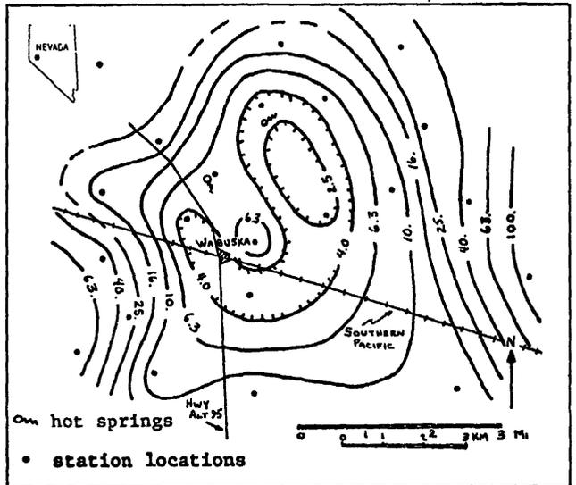
Fig. 3 Audio-magnetotelluric apparent resistivity map at 7.5 hertz, Wabuska, Nevada KGRA, logarithmic contours in ohm-meters.
